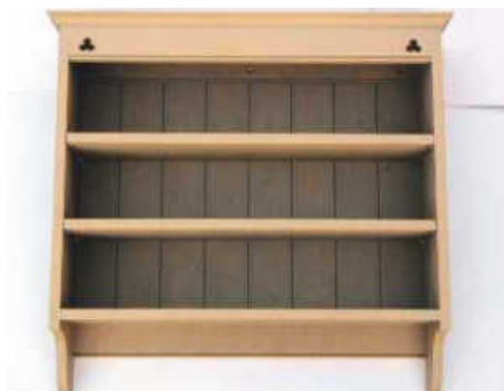
STEP 24. Check the unit is fixed solidly before loading up shelves. Use 5.0mm screws for fixing
